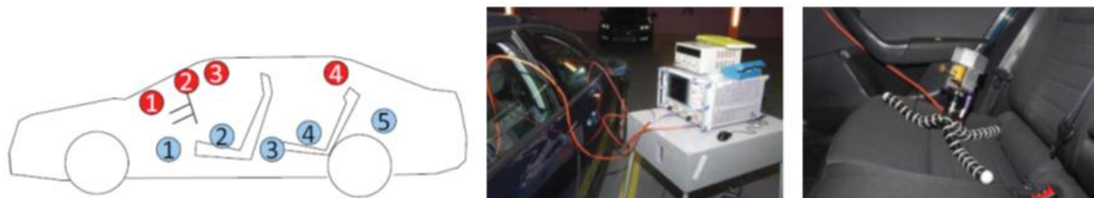
Figure 2: Antenna position of the RX (red) and TX (blue) in the vehicle and the measurement setup.
