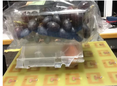
Fig. 1: Illustration of one of the test setups carried out using the UWB sensors in a smart fridge scenario, where there are grapes placed over the eggs in this test scenario.
